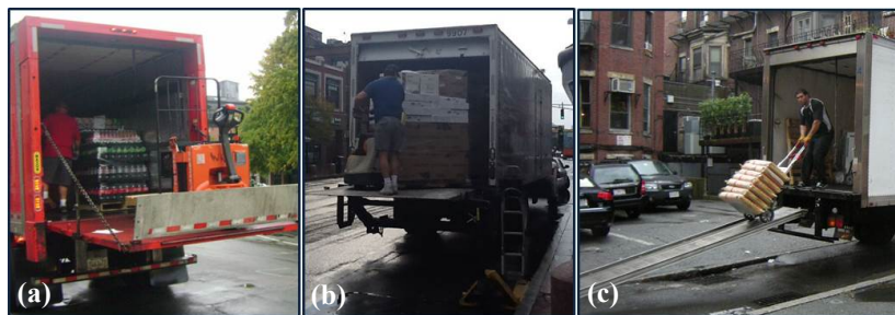
Figure 8: Support equipment – liftgates (a, b) and unloading ramp (c)
